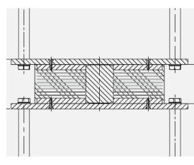
Elastomeric lead rubber bearing with inner lead core and anchor plates with shear dowels for anchoring in the concrete.
