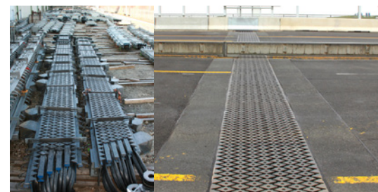
On the left: Ready-for-delivery expansion joint with 4 profiles at MAURER in Munich.
