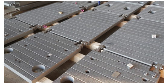
Mega-MMBS elements before transport to Hamburg. Clearly visible: various recesses to accommodate the anchoring.
