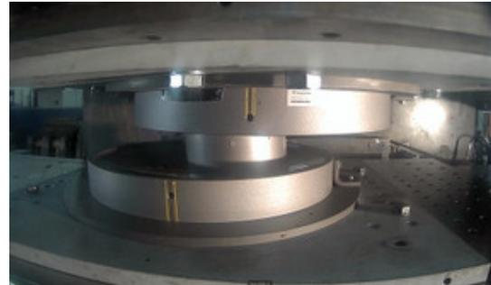
Prototype testing of the SIP® bearing at EUCENTRE Pavia.
