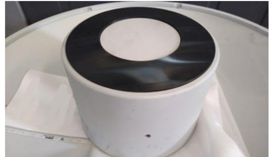
Unusual insight: a puck, the centre piece of a SIP®-Bearing. The photo was taken during the overhaul of a prototype bearing following testing.
