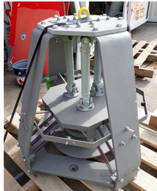
The Tuned Mass Damper (TMD) consists of an octagonal pendulum mass hanging on three rods with Cardan joints, four stacked friction plates below the pendulum mass, and tuning springs installed between the rack and the pendulum mass for natural frequency tuning. The special shape of the TMD rack allows the TMD to be installed horizontally in the Red Stick, which is inclined at an angle of 20 degrees.
