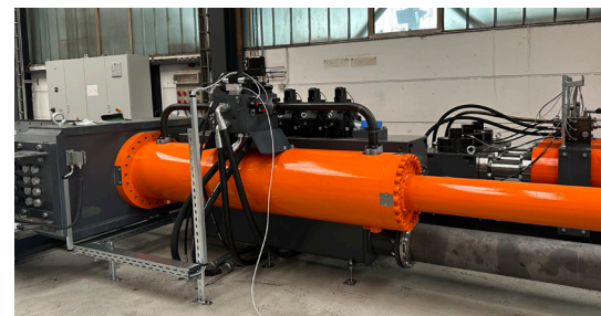
The large hydraulic actuator controls the movements of the testing press with high power and precision – a key requirement for large test specimens and demanding load simulations.
