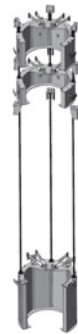
The three tuned mass dampers (TMDs) arranged on top of each other.
