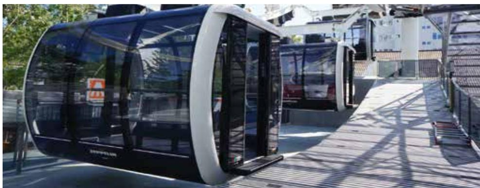
27 Zeppelin cabins, fully air-conditioned, for up to 16 passengers, spin their rounds above Munich
