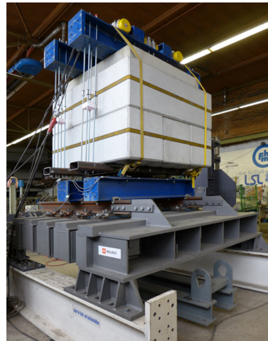
Test set up for the 10-km sliding displacement test and a load fatigue test. There was no wear in the moving parts of the Guided Cross-Tie.
