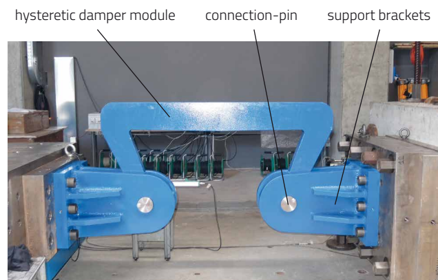
Fig. 2: Components of a MANTIS® device
