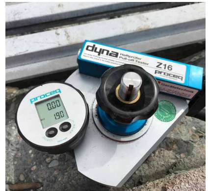
Measurement of adhesion
