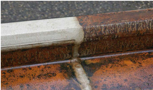
Fig. 1 – Upper part of the claw - non-corrosive steel
